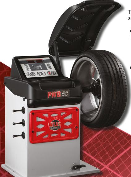
The Fast & Easy Split function (FES) makes hiding adhesive weights behind the spokes a breeze, and the Opposite Weight Function (OWF) allows an operator to change the weight application position from 12 o'clock to 6 o'clock for convenient access when applying adhesive weights.
