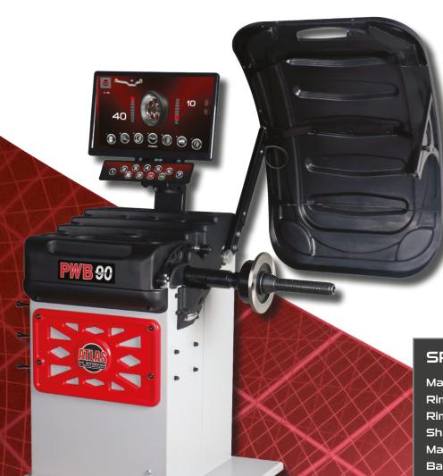
This machine offers Super Automatic 3D Data Entry via a single data entry gauge for offset and diameter, and touchless sonar for rim width (no more old-fashioned measuring arms). Using the weight placement arm, the user can choose the most convenient location to put the weights, and a laser will guide the operator back to the exact location after the spin cycle, eliminating any possibility for human error and ensuring first time zero/zero results.
